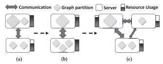
**Figure 1.** PageRank elasticity management example: **(a)** The initial placement of graph partitions overloads the top server which calls for partition migration. **(b)** Once migration is performed, the bottom server becomes congested. **(c)** With both servers reaching their maximum capacity, PLASMA migrates to a new server to split the load of the bottom one.
