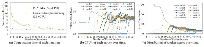
**Figure 8.** PageRank dynamic resource allocation. PLASMA achieves the same application-level performance with 12 servers in comparison with the conservative provisioning case using 16 servers (with one worker per vCPU).
