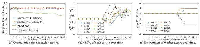
**Figure 7.** PageRank dynamic workload balance. PLASMA achieves 24% faster iteration times after initial automated balancing. (In **(b)** and **(c)**, each server is busy reading data in the early re-distributions.)
